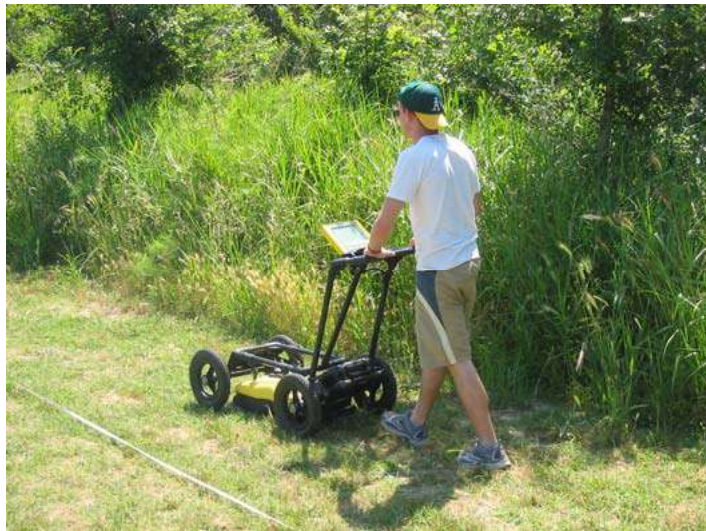
Ground Penetrating Radar (GPR)
