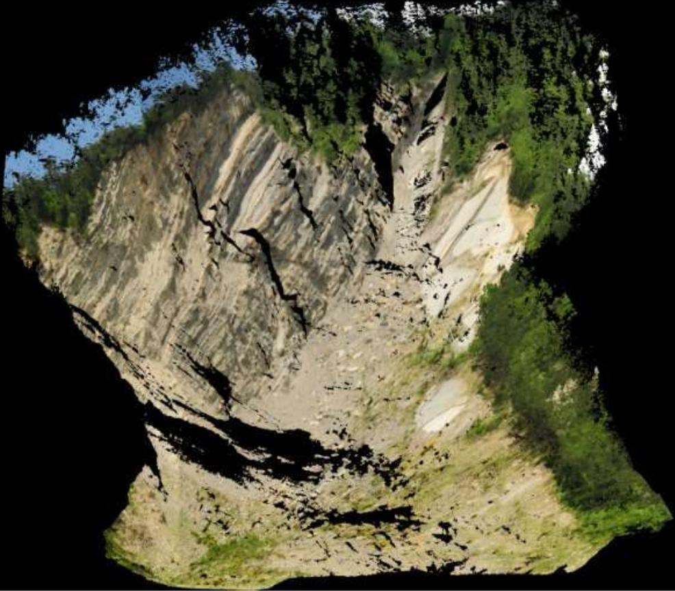
*3D model in real colors retrieved by a Terrestrial Laser Scanner survey of a rock scarp.*
