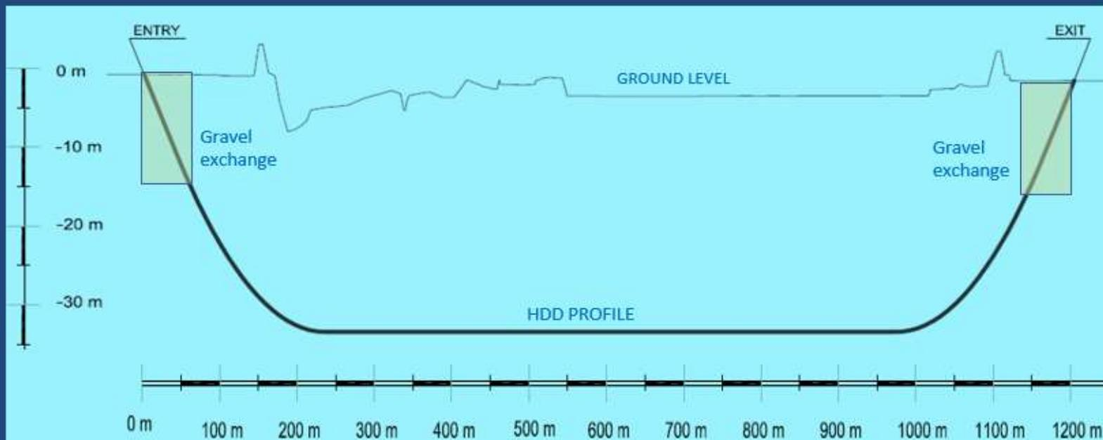
The HDD profile has the following characteristics:
